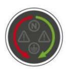
Simultaneous illumination of "rotating field left" and "rotating field right" (also in combination with any other symbol) indicates an error, which has to be checked by a qualified electrician.
